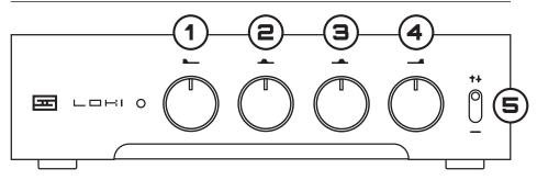
**1 Bass Adjustment.** (20Hz) Turning the knob clockwise increases bass, turning it counter-clockwise decreases bass. Like all the adjustments on Loki, it has a gradual effect when first turned off of the center position, for subtle adjustments.
